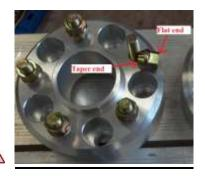
H. Get your socket & add Loctite to the 5 studs on the spacer. Install the rim/wheel & now use the new nuts, making sure they are flip to the proper end, as describe (above pic). Torque the nuts to 65 ft. lbs for the rim in the same 3 steps as above.
