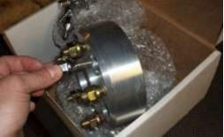
Now is a good time to test fit the spacer to the Axle & then to the wheel rim. The spacer should make full contact to the axle, it's much easier to sort any problems without having anything bolted down.
